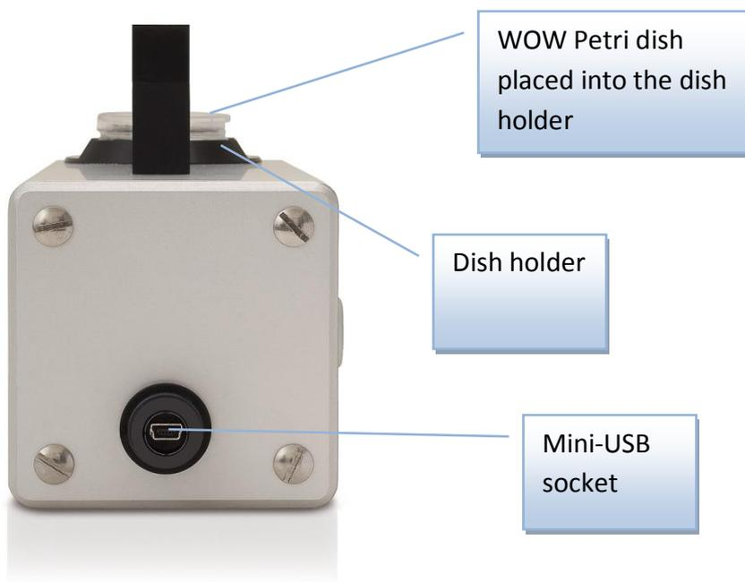
Before first use, disinfect the external surface and the USB cable with 96% ethanol. Following wiping, let the ethanol evaporate, or further wipe with distilled water inside a laminar hood before placing the unit(s) into the incubator. Disinfection is also possible with other approved solutions to be used inside the incubators, complying with current rules and regulations.
