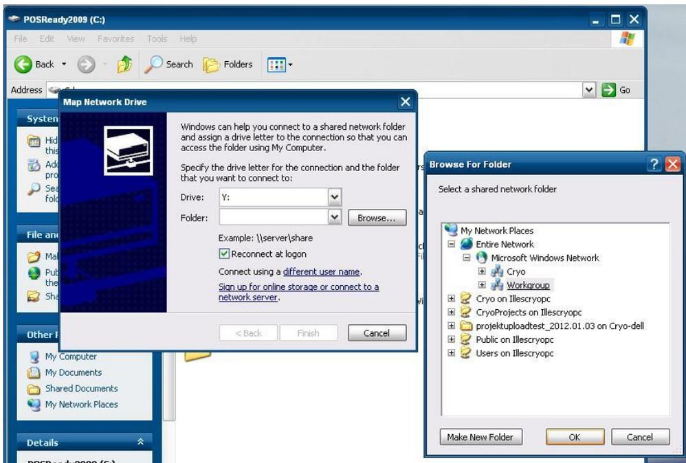
The Analyzer software now can be started and the project can be opened as described previously in this chapter. The shared folder will be available as a local drive (in accordance to the drive letter set in the „Map network drive” setup) after clicking on the „Open” button.
