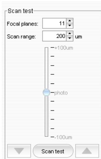
This function can help in finding the best scan settings for the Settings menu / Time-lapse defaults (see details in Chapter 3.2.6. „Scanning” and 3.2.7. „Settings / Time-lapse defaults”).
