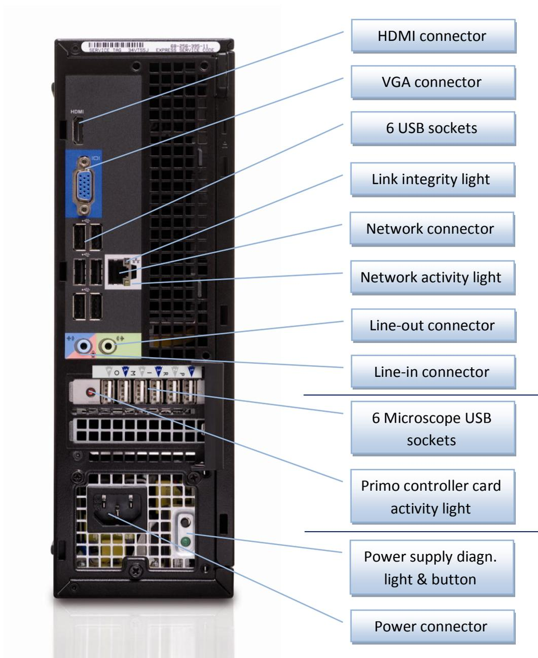
The Controller Unit is equipped with Windows XP Embedded POS-Ready operating system, which runs the Capture and Analyzer software, and has 500 GB storage capacity.
