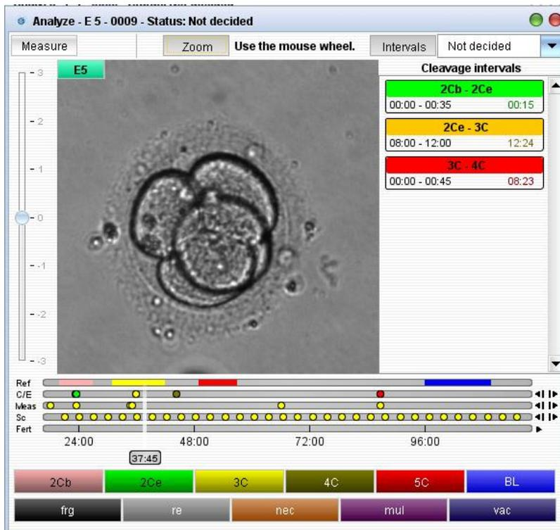
Regarding to the reference values and the tolerance rate, set in the „Settings“, the legend of the given interval can be seen in the tones between green (the cleavage interval of the embryo is within the reference values), orange (out of the reference values, but within the tolerance rate), and red (out of the reference values and the tolerance rate).
