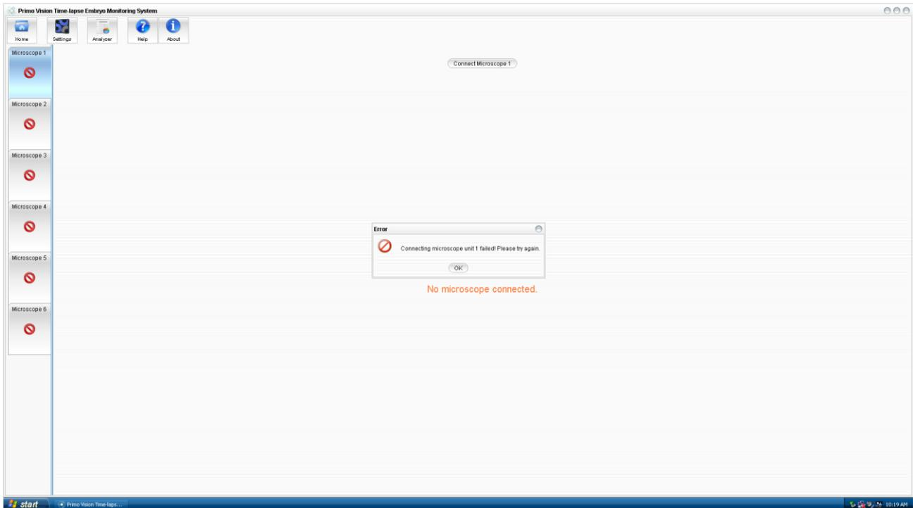
In this case check the USB plug and the number of the Microscope, close the pop-up window and click on „Connect Microscope 1” button again.
