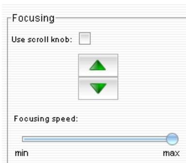
Alternatively 3D mouse can be used for focus settings. After clicking on „Use scroll knob”, twist the 3D mouse gently to find the best focal plane.
