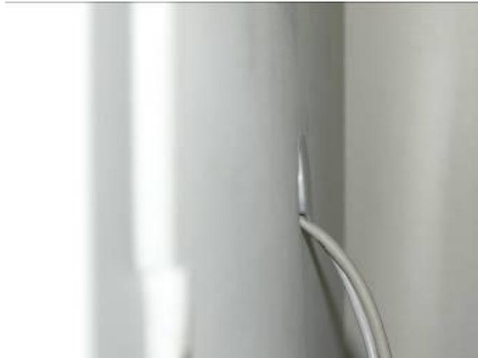
Some incubators do not have a factory made opening on the side/back. In this case, the USB cables may be led through the side of the incubator door.
