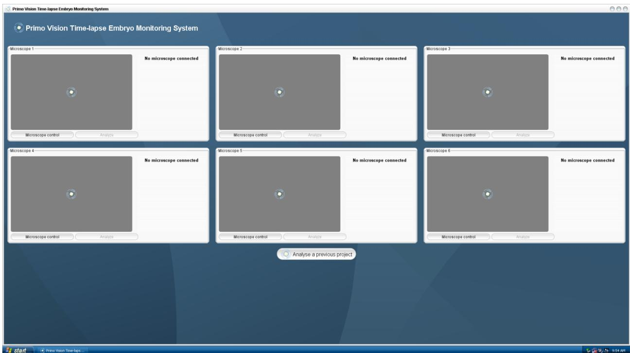
To start a project with the first Microscope, click on the „Microscope control” button below the image of the given Microscope. On the next screen click on „Connect Microscope 1” button.
