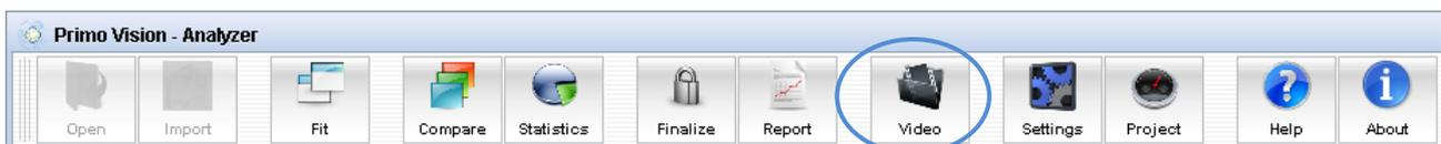
By clicking on the „Video” button on the upper part of the screen, a video file can be created of the time-lapse photo series. If pressing this button, a pop-up window will appear, where the video size (normal or small), output format (AVI or MOV), frame rate (slow, normal or fast) and image type (well or embryo view) can be set. Videos of individual embryos can be created by clicking on the checkboxes of the embryos or by clicking on „Select all”, or a video with all the embryos in the
