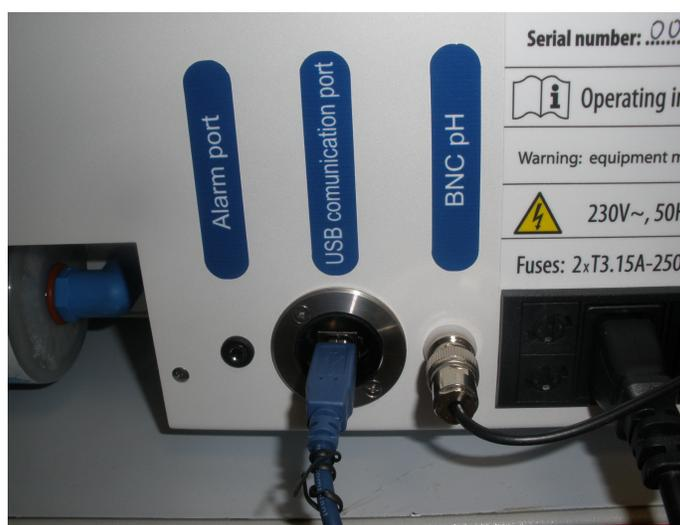
**Figure 10. pH Probe Connected To the BNC**
